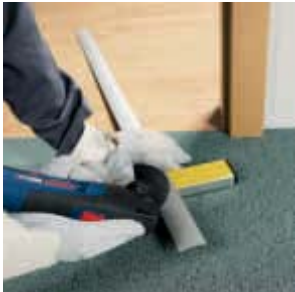
Cutting moldings to length with ease, e.g. aluminium floor cover strip.
