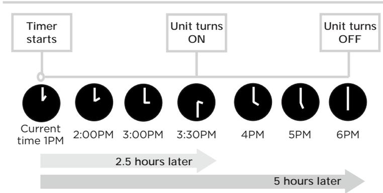
Example: If current time is 1:00PM, to set the timer as above steps, the unit will turn on 2.5h later (3:30PM) and turn off at 6:00PM.:
