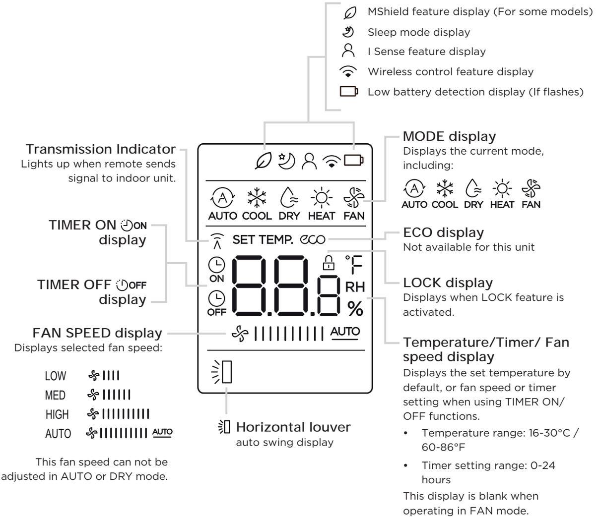
This fan speed can not be adjusted in AUTO or DRY mode.
