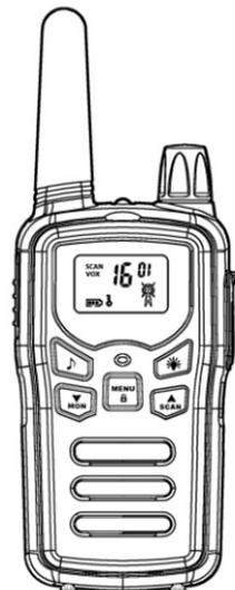
This set includes 2 walkie-talkie units: these are communication devices that operate on mobile radio frequencies. They have 8(Europe)/ 22(US) channels as well as a back-lit LCD screen, enabling you to communicate over several kilometers free-of-charge (up to 5miles in open areas).
